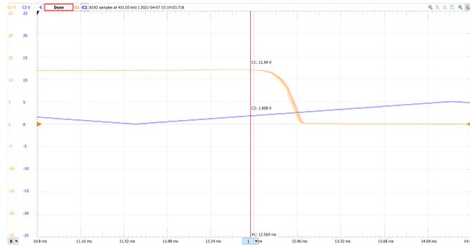
Fig. 40. Measurement of  $V_{t0}$  for transistor 3.
