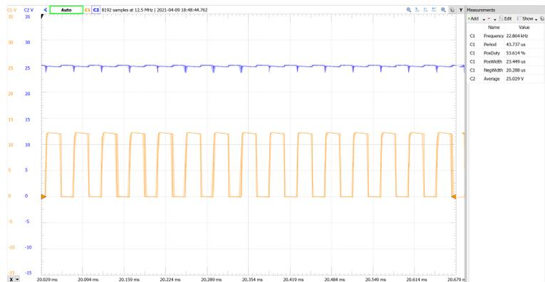
Fig. 42. Measurements taken of combined boost converter and astable multivibrator circuits.
